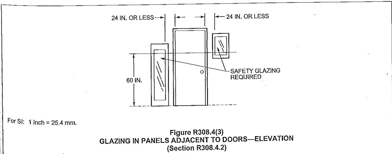
Section R308.4.3. Under this section, all four stated conditions must occur before safety glazing is required. These conditions are as follows:
